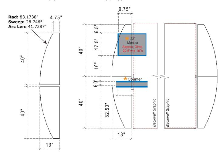
**NOTE:** These dimensions are for graphic layout purposes. Graphic needs to be cut and test fitted to Sacagawea frame.
