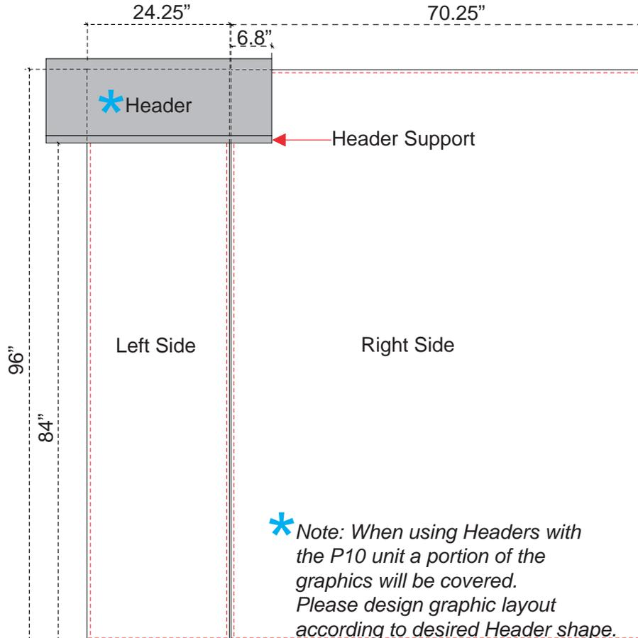
NOTE: These dimensions are for graphic layout purposes. Graphic needs to be cut and test fitted to frame.
