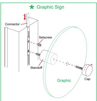
Slide connector into groove of extrusion. Tighten set screw to secure in place. Screw standoff into connector. Place graphic between standoff and cap then secure graphic to standoff, using cap.
