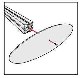
Base Plate & Extrusion Connection
