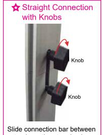
extrusions, then turn knobs clockwise to tighten lock.
